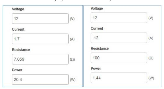
Ohm's Law was used to calculate the load value (delta) for both a LED and load resistor in the circuit to duplicate the current draw of the incandescent stop lamp.
