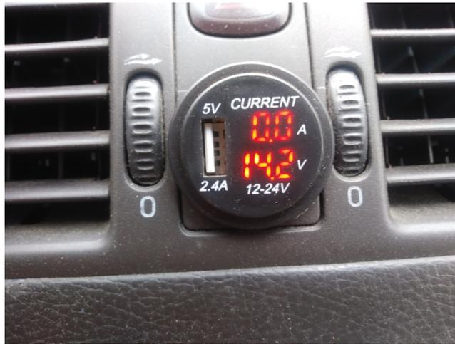
Sure'nuf, each time the charging system failure warning appeared, the alternator output was 13.8 volts. Cutting the engine and restarting returned the output to 14.+ volts. The nominal voltage of a fully charged 12 volt battery is 12.6 volts. So, the alternator had not failed, but continued to push current into the battery. The ECU's message was erroneous.
