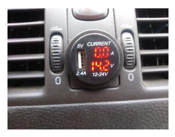
Sure'nuf, each time the charging system failure warning appeared, the alternator output was 13.8 volts. Cutting the engine and restarting returned the output to 14.+ volts. The nominal voltage of a fully charged 12 volt battery is 12.6 volts. So, the alternator had not failed, but continued to push current into the battery. The ECU's message was erroneous.
