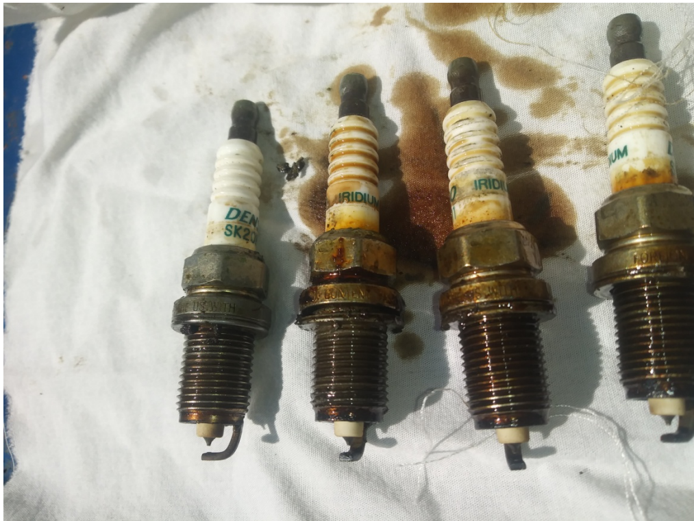
Three Bank 1 plugs submerged in oil
