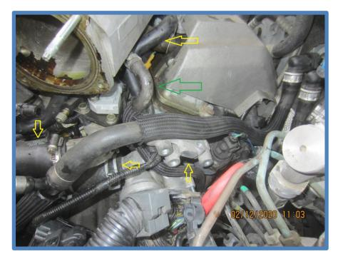
Remove the two fasteners attaching the starter to the bell housing.
