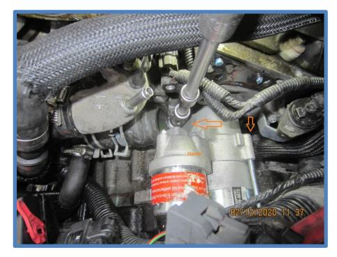
Lift starter, turn sideways, and push wire harnesses aside and carefully lift it out. The extraction process shouldn't take more than 60 seconds. I used a bungee cord to lift and hold the wire harness and hoses aside to gain clearance.
