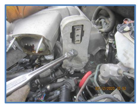
Carefully remove water (yellow arrow) and vacuum (green arrow) hoses and water by pass device. Be ABSOLUTELY certain to mark the PCV vacuum hose to prevent accidental connection of a water line to the manifold intake. If incorrectly reconnected, you'll pump coolant into the engine upon restart and push coolant into the PVC system. Not good!
