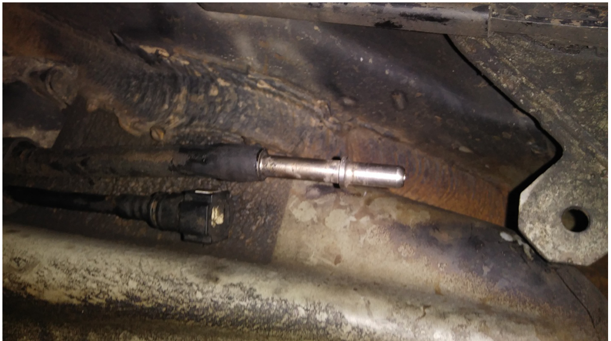
Disconnected fuel supply lines from tank at rear of engine cradle
