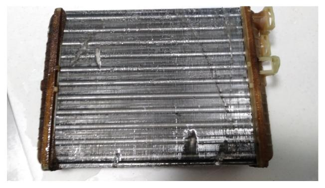
Although the fins are crumpled, this is a good working donor unit. The fins are groomed and restored by using a dull single edge razor blade to separate vanes. This is necessary to maximize air flow, heat transfer, through the heater core.
