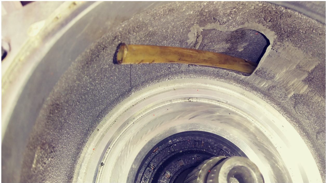
View of Haldex Clutch Pack Chamber and Oil Fill Tube
