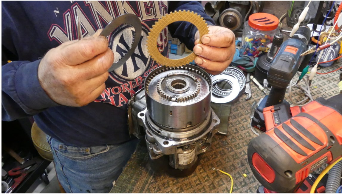
Haldex Has Alternating Clutch Disks and Plates.
