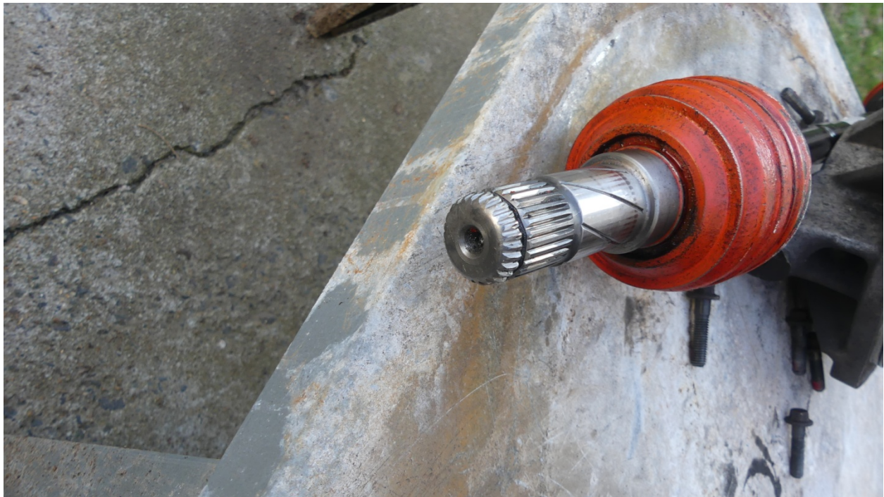
Spline Tip Misaligned/Twisted by Axle Gear Torque.
