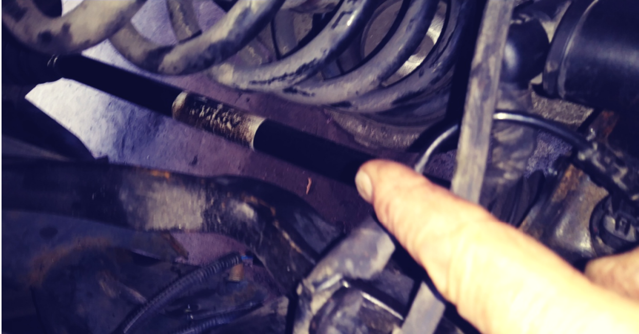
Pointing to Replacement Right Axle
