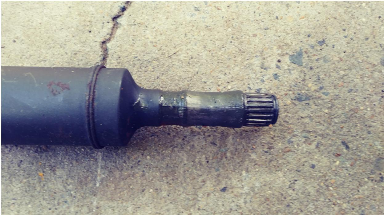
The donor driveshaft spline (above). There is a CV joint at both ends. Since one was needed, I have a spare CV coupler. So a task that could have become labor intensive was simplified by replacing the worn part as opposed to the entire driveshaft. I do not understand why this component is not offered as a replacement item. If you can use the other driveshaft CV coupler, contact me by email.
