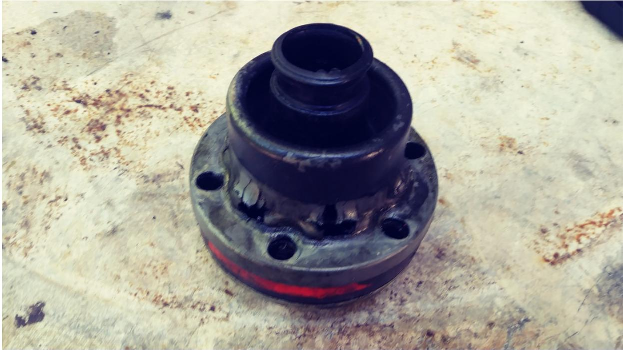
The donor CV coupler was installed in reverse order. Placing an impact socket larger than the driveshaft spline over the CV coupler, I tapped it in place with a ball peen hammer and replaced the retaining clip. I filled the rear dust cover with grease and placed it over the coupler and tie wrapped the boot to the driveshaft spline.
