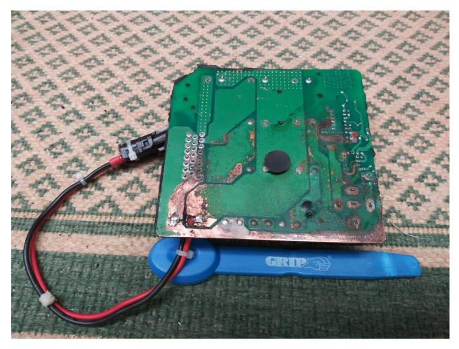
In above picture, the microprocessor controller is on right side and power is inserted at the lower left corner. I cleaned the traces, repaired damage, installed a power pigtail and tested all solder joints for continuity. I was fortunate the microprocessor was not compromised. If it had been, another could be ordered by placing its part number, located on the upper surface, on the Internet. I did this, and found them available along with a schematic showing the companion components.
