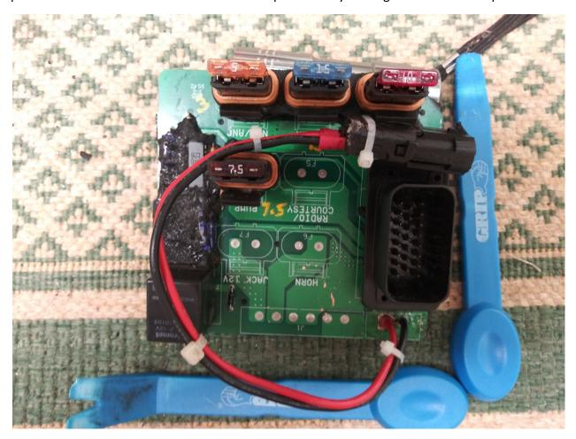
The board separated from the tray easily. I observed water infiltrated the potting tray along the vertical edges in cracks between the tray and the epoxy. Moisture worked its way beneath the board and corroded solder joints, compromised traces, breaking circuits and the resulting corrosion caused a short, which burned the board.
