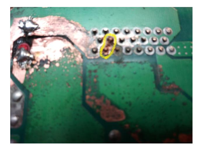
The repaired circuit board awaits installation. I plan to seal the bottom with a clear spray urethane; then, place the board in the tray and seal it by placing a bead of silicone along the edge of the circuit board and the tray.
